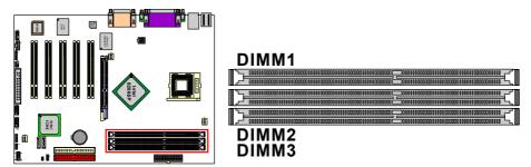
The PX865PEL-800 provides three DIMM sockets which support 184-pin DDR DIMM modules with a total memory capacity of up to 2 GB. Each DIMM socket is capable of using a memory module containing up to 1 GB. Further limitations and recommendations are listed below:
